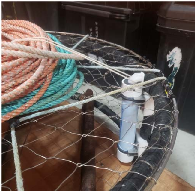
Vertical installation on a crab trap with the TR4RT inside the trap.
